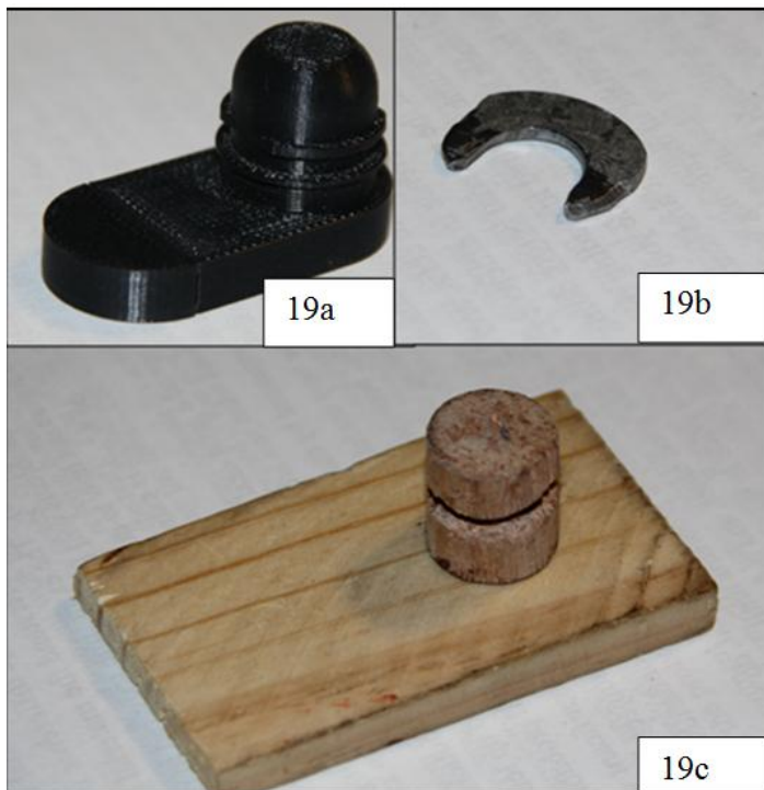
Figure 19: 19a) A display of the enlarged version of the magnetic secured housing. 19b) The ferrous slider model was made by grinding down an iron washer. 19c) Enlarged model of the abutment. The wood block simulates the mastoidal base of the abutment while the cork cylinder models the abutment itself.
