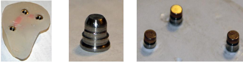
Figure 2: (Left) O-ring system within mock prosthetic. (Center) Outside of a single O-ring magnetic cap. (Right) 3 abutments that are implanted into a clay base.
