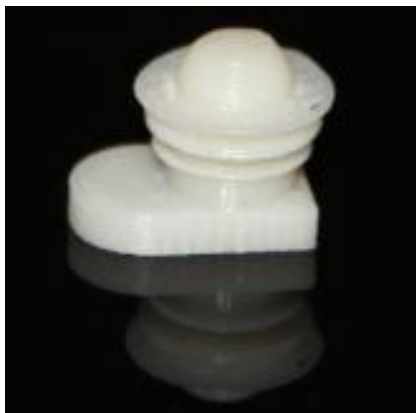
Figure 16: Actual Size Prototype. Note the large rings towards the top used to hold the housing in the prosthetic's silicone.
