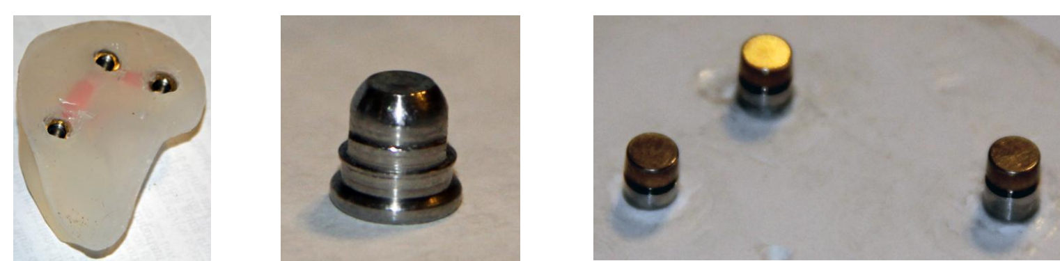
Figure 1: (Left) O-ring system within mock prosthetic. (Center) Outside of a single O-ring magnetic cap. (Right) 3 abutments that are implanted into a clay base.
