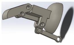
**Figure 1.** When a patient bends their finger, the rightmost link hits the distal phalanx and forces a bend in the prosthetic distal end. By manipulating the relative sizes of the links, our client can change the force necessary to initiate prosthetic movement and the range of motion achievable by the total finger system.
