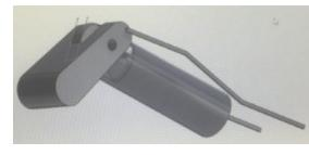
**Figure 2.** The wires depicted in this design attaches to a ring just below the proximal joint of the residuum of the finger. The rod will be directly attached to a cap covering the residuum. As the proximal joint bends, the force from the wires creates a moment in the lever acting as the distal phalanx. This leverage causes the device to bend downward, and the subsequent extension of the proximal joint will in turn cause the lever to extend.
