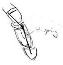
**Figure 3.** This design incorporates both a push/pull design centered on a ring the patient wears and a lever mechanism resting on the anterior surface of the amputated finger. By use of a moment arms the device will be able to flex based on the patient's articulation of their finger. The design features a built in spring to assist with extension of the finger following flexion.
