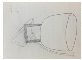
**Figure 4.** This design uses a push/pull system to control the flexion and extension of the prosthesis. As the lever on the bottom of the prosthesis is pushed to the left, it causes a moment imbalance at the two pins holding the mechanism onto the anchor frame. As the lever on the bottom is retracted back to the right, these moment imbalances reverse, causing extension of the joint.
